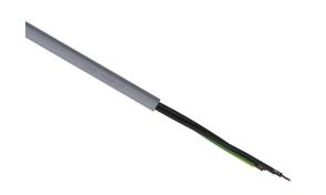
LUTZE SUPERFLEX continuous flexing control cable, unshielded, 3 conductors (includes ground), 16 AWG (1.50mm2), bare copper, TPE conductor insulation material, black with white numbers and green/yellow ground, PVC jacket, gray, cut to length.
