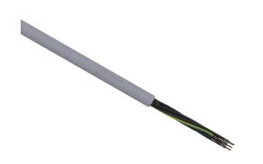
LUTZE SUPERFLEX continuous flexing control cable, unshielded, 7 conductors (includes ground), 14 AWG (2.50mm2), bare copper, TPE conductor insulation material, black with white numbers and green/yellow ground, PVC jacket, gray, cut to length.
