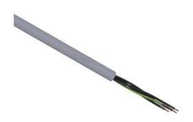
LUTZE SUPERFLEX continuous flexing control cable, unshielded, 5 conductors (includes ground), 14 AWG (2.50mm2), bare copper, TPE conductor insulation material, black with white numbers and green/yellow ground, PVC jacket, gray, cut to length.
