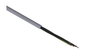
LUTZE SUPERFLEX continuous flexing control cable, unshielded, 4 conductors (includes ground), 14 AWG (2.50mm2), bare copper, TPE conductor insulation material, black with white numbers and green/yellow ground, PVC jacket, gray, cut to length.
