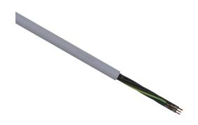
LUTZE SUPERFLEX continuous flexing control cable, unshielded, 7 conductors (includes ground), 12 AWG (4mm2), bare copper, TPE conductor insulation material, black with white numbers and green/yellow ground, PVC jacket, gray, cut to length.
