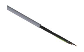
LUTZE SUPERFLEX continuous flexing control cable, unshielded, 4 conductors (includes ground), 12 AWG (4mm2), bare copper, TPE conductor insulation material, black with white numbers and green/yellow ground, PVC jacket, gray, cut to length.
