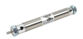
NITRA pneumatic cylinder, non-repairable, 7/8in bore, 1/4in rod diameter, 4in stroke, double acting, magnetic piston, double end mount.
