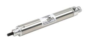
NITRA pneumatic cylinder, non-repairable, 7/8in bore, 1/4in rod diameter, 3in stroke, single acting, rear pivot mount.
