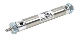
NITRA pneumatic cylinder, non-repairable, 7/8in bore, 1/4in rod diameter, 3in stroke, double acting, double end mount.
