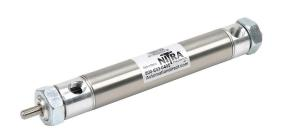
NITRA pneumatic cylinder, non-repairable, 7/8in bore, 1/4in rod diameter, 3in stroke, double acting, magnetic piston, double end mount.
