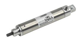
NITRA pneumatic cylinder, non-repairable, 7/8in bore, 1/4in rod diameter, 2in stroke, single acting, rear pivot mount.
