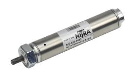
NITRA pneumatic cylinder, non-repairable, 7/8in bore, 1/4in rod diameter, 2in stroke, single acting, front nose mount.
