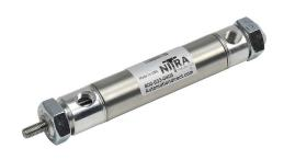
NITRA pneumatic cylinder, non-repairable, 7/8in bore, 1/4in rod diameter, 2in stroke, double acting, double end mount.
