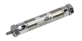
NITRA pneumatic cylinder, non-repairable, 7/8in bore, 1/4in rod diameter, 2in stroke, double acting, magnetic piston, double end mount.
