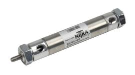
NITRA pneumatic cylinder, non-repairable, 7/8in bore, 1/4in rod diameter, 2in stroke, double acting, magnetic piston, double end mount.
