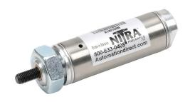
NITRA pneumatic cylinder, non-repairable, 7/8in bore, 1/4in rod diameter, 1in stroke, single acting, front nose mount.
