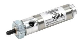
NITRA pneumatic cylinder, non-repairable, 7/8in bore, 1/4in rod diameter, 1in stroke, double acting, front nose mount.
