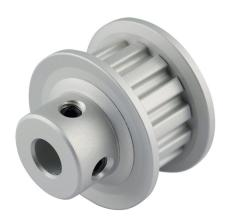
Sung-II Machinery timing pulley, aluminum, 1/5in XL pitch, 14 tooth, 0.891in pitch diameter, 1/4in bore, hub with flanges. For use with 3/8in wide belt.
