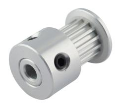
Sung-Il Machinery timing pulley, aluminum, 0.08in MXL pitch, 14 tooth, 0.357in pitch diameter, 1/8in bore, oversize hub with flange. For use with 1/4in wide belt.
