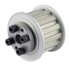
Sung-Il Machinery timing pulley, aluminum, 3/8in L pitch, 14 tooth, 1.671in pitch diameter, 3/8in bore, no hub with flanges. For use with 1in wide belt. QD bushing included.
