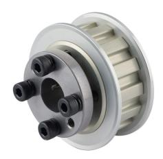
Sung-Il Machinery timing pulley, aluminum, 3/8in L pitch, 14 tooth, 1.671in pitch diameter, 1/2in bore, no hub with flanges. For use with 1/2in wide belt. QD bushing included.
