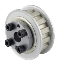
Sung-Il Machinery timing pulley, aluminum, 3/8in L pitch, 14 tooth, 1.671in pitch diameter, 3/8in bore, no hub with flanges. For use with 1/2in wide belt. QD bushing included.
