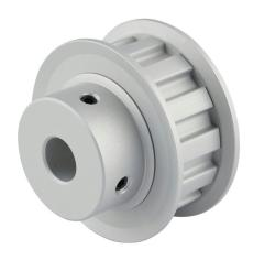
Sung-Il Machinery timing pulley, aluminum, 3/8in L pitch, 13 tooth, 1.552in pitch diameter, 3/8in bore, hub with flanges. For use with 1/2in wide belt.
