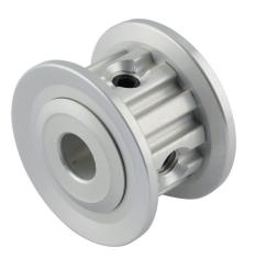
Sung-Il Machinery timing pulley, aluminum, 1/5in XL pitch, 12 tooth, 0.764in pitch diameter, 1/4in bore, no hub with flanges. For use with 3/8in wide belt.
