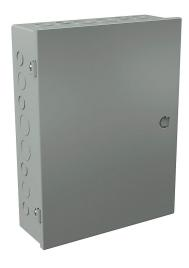
Wiegmann enclosure, NEMA 1, 16 x 12 x 4in (HxWxD), wall mount, with knockouts, carbon steel, ANSI 61 gray, powder coat finish, single-door, integral snap-tight latch.
