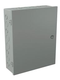
Wiegmann enclosure, NEMA 1, 15 x 12 x 4in (HxWxD), wall mount, with knockouts, carbon steel, ANSI 61 gray, powder coat finish, single-door, integral snap-tight latch.
