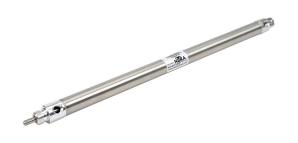
NITRA pneumatic cylinder, non-repairable, 3/4in bore, 1/4in rod diameter, 12in stroke, double acting, magnetic piston, rear pivot mount.
