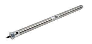
NITRA pneumatic cylinder, non-repairable, 3/4in bore, 1/4in rod diameter, 12in stroke, double acting, front nose mount.
