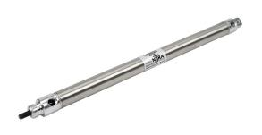
NITRA pneumatic cylinder, non-repairable, 3/4in bore, 1/4in rod diameter, 10in stroke, double acting, rear pivot mount.
