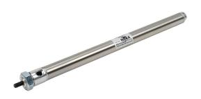
NITRA pneumatic cylinder, non-repairable, 3/4in bore, 1/4in rod diameter, 10in stroke, double acting, front nose mount.
