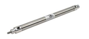
NITRA pneumatic cylinder, non-repairable, 3/4in bore, 1/4in rod diameter, 8in stroke, double acting, magnetic piston, rear pivot mount.
