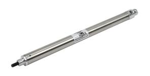
NITRA pneumatic cylinder, non-repairable, 3/4in bore, 1/4in rod diameter, 6in stroke, single acting, rear pivot mount.
