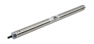
NITRA pneumatic cylinder, non-repairable, 3/4in bore, 1/4in rod diameter, 6in stroke, single acting, front nose mount.
