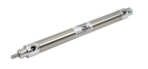
NITRA pneumatic cylinder, non-repairable, 3/4in bore, 1/4in rod diameter, 6in stroke, double acting, magnetic piston, rear pivot mount.
