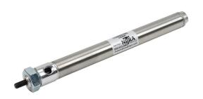
NITRA pneumatic cylinder, non-repairable, 3/4in bore, 1/4in rod diameter, 6in stroke, double acting, front nose mount.
