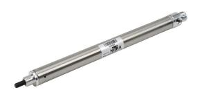
NITRA pneumatic cylinder, non-repairable, 3/4in bore, 1/4in rod diameter, 5in stroke, single acting, rear pivot mount.
