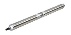
NITRA pneumatic cylinder, non-repairable, 3/4in bore, 1/4in rod diameter, 5in stroke, single acting, front nose mount.
