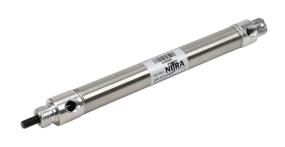
NITRA pneumatic cylinder, non-repairable, 3/4in bore, 1/4in rod diameter, 5in stroke, double acting, rear pivot mount.
