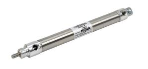
NITRA pneumatic cylinder, non-repairable, 3/4in bore, 1/4in rod diameter, 5in stroke, double acting, magnetic piston, rear pivot mount.
