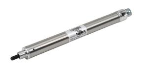
NITRA pneumatic cylinder, non-repairable, 3/4in bore, 1/4in rod diameter, 4in stroke, single acting, rear pivot mount.
