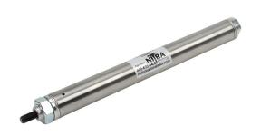
NITRA pneumatic cylinder, non-repairable, 3/4in bore, 1/4in rod diameter, 4in stroke, single acting, front nose mount.
