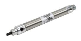
NITRA pneumatic cylinder, non-repairable, 3/4in bore, 1/4in rod diameter, 4in stroke, double acting, rear pivot mount.
