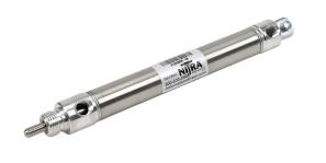
NITRA pneumatic cylinder, non-repairable, 3/4in bore, 1/4in rod diameter, 4in stroke, double acting, magnetic piston, rear pivot mount.
