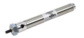
NITRA pneumatic cylinder, non-repairable, 3/4in bore, 1/4in rod diameter, 4in stroke, double acting, front nose mount.
