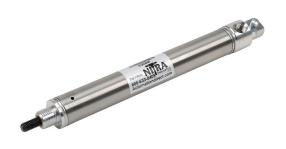
NITRA pneumatic cylinder, non-repairable, 3/4in bore, 1/4in rod diameter, 3in stroke, single acting, rear pivot mount.
