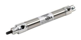
NITRA pneumatic cylinder, non-repairable, 3/4in bore, 1/4in rod diameter, 3in stroke, double acting, rear pivot mount.
