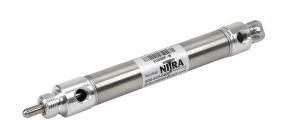
NITRA pneumatic cylinder, non-repairable, 3/4in bore, 1/4in rod diameter, 3in stroke, double acting, magnetic piston, rear pivot mount.
