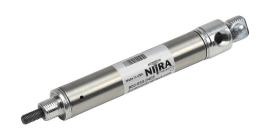
NITRA pneumatic cylinder, non-repairable, 3/4in bore, 1/4in rod diameter, 2in stroke, single acting, rear pivot mount.
