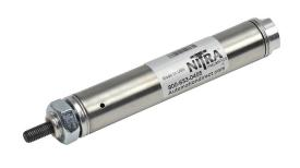
NITRA pneumatic cylinder, non-repairable, 3/4in bore, 1/4in rod diameter, 2in stroke, single acting, front nose mount.
