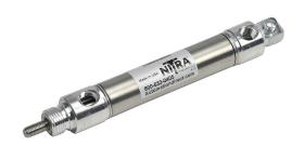
NITRA pneumatic cylinder, non-repairable, 3/4in bore, 1/4in rod diameter, 2in stroke, double acting, magnetic piston, rear pivot mount.
