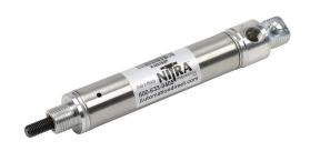
NITRA pneumatic cylinder, non-repairable, 3/4in bore, 1/4in rod diameter, 1-1/2in stroke, single acting, rear pivot mount.
